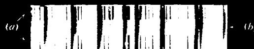
FIG. 4. Examples of line and band emission spectra. The line spectrum, marked (a), is part of the spectrum emitted by the iron arc; and the band spectrum, marked (b), is emitted by the diatomic molecule antimony fluoride (SbF). The line spectrum is superimposed on the band spectrum.
